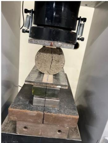
*Figure 3. Splitting tensile strength test*
